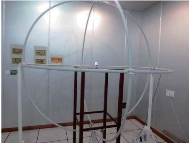
Figure 3 Radiated Magnetic Field emission test setup
