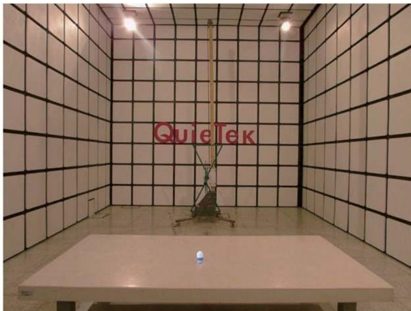
Figure 3 Radiated Magnetic Field emission test setup
